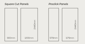
**Proclick technology** has been engineered to create a mechanical locking system that provides seamless, almost invisible joints. Installation is made easy through the click design which allows panels to be located quickly and easily into place, eliminating the use of joining trims.
